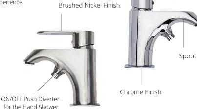
NOTE: This faucet is designed to be installed through: G.W: 7.75 kg/ 17 lbs., 2-1/2" diameter hole for faucet, 1/3" diameter hole for mounting rods, 7/8" diagonal hole for hand shower
