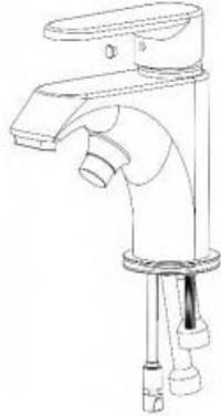
Step.2 Use an Allen wrench to remove the handle Screw.
