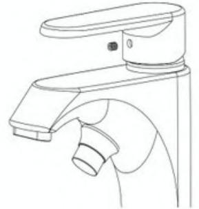
Step.3 Take out the handle and remove the brass escutcheon
