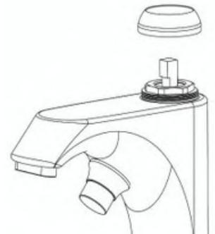
Step.5 Remove the cartridge and replace it with new piece.
