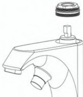
Step.4 Use a wrench to unscrew the pressure cap.
