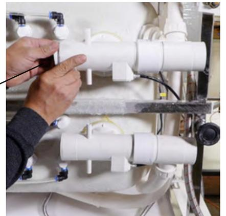
T-Type four (4) 2" drain ports
