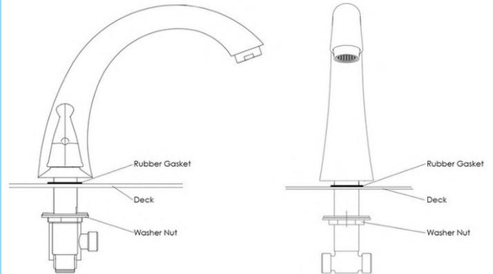
**2.** Unscrew the washer nut and place the rubber gasket and spout above the deck. After, secure the washer nut from underneath the deck.
