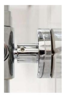
The The shower column is attached to the wall with either a short or long pipe connector. The long pipe can range between 9 3/4" to 10 3/4". The short pipe can range between 2 1/4" to 3 1/4". These two images show a short pipe connector.
